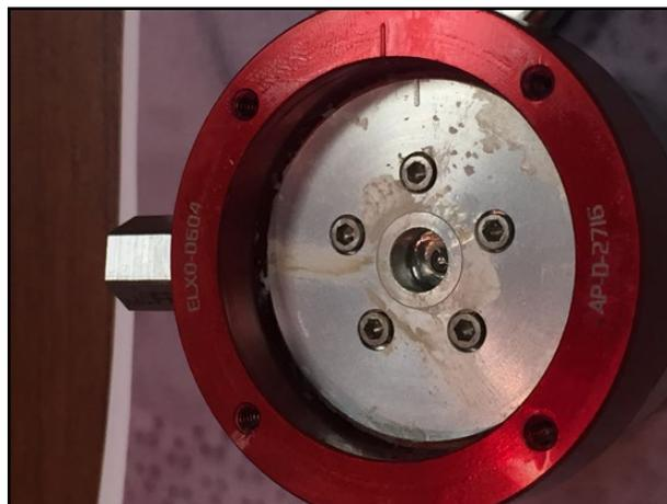
Figure 2 – Actuator contamination
