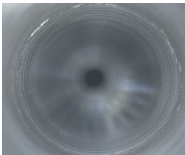
■ Figure 10C: Initial surface finish of fitting taper
