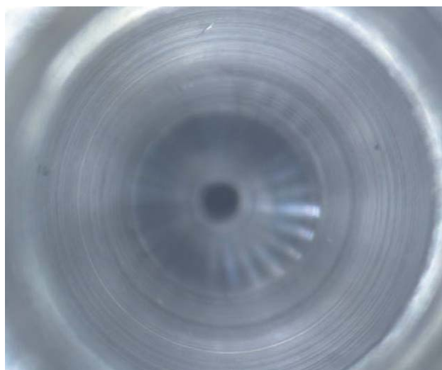
■ Figure 10C: Initial surface finish of fitting taper
